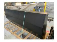
For the new gas tank, Tony decided to have it built using heavier gauge aluminum and coated it for extra corrosion protection.
